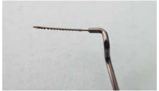
Figure 1. The SCE mounted on 0.2 mm thick microprobe having curvature as of SC. The distal end of the microprobe had certain angulations to facilitate device insertion into SC
